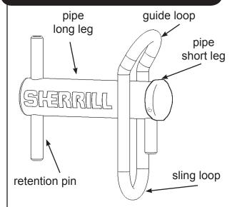
INSPECT: Prior to use, always inspect Portawrap and supporting lines for damage or excessive wear. Replace materials that show signs of excessive wear.
